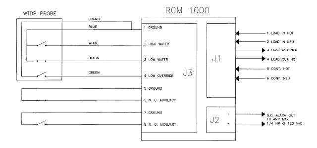
If the N.C. Auxiliary input is not used, terminals J3-5 and J3-6 must be jumpered together.
